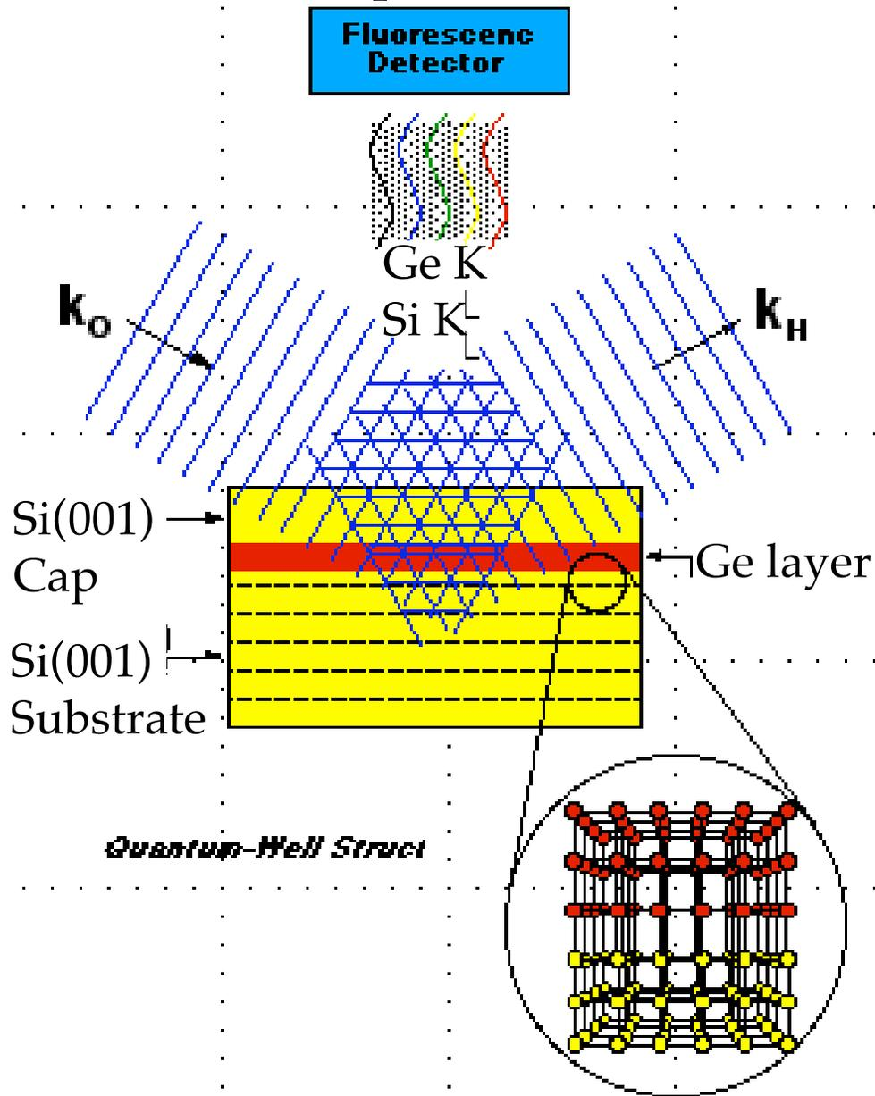
Can measure strain down to the level of 1 atomic layer.
