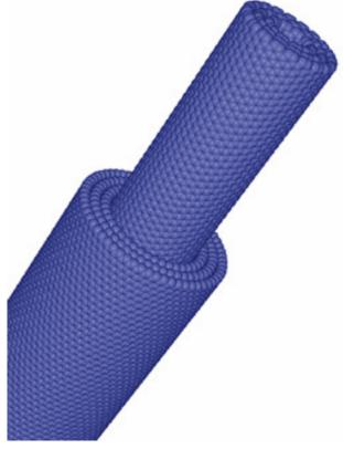
The controlled and reversible telescopic extension of MWNTs as shown in the computer graphic [above], could lead to virtually frictionless nanoscale linear bearings and constant-force nanosprings.
